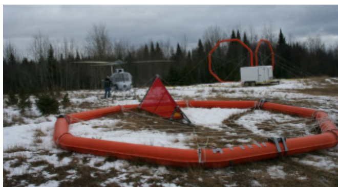
Figure 3: ZTEM z-axis receiver and ground-based prototype reference coils from field tests in northern Ontario, Canada in 2006 (after Lo and Kuzmin, 2008).
