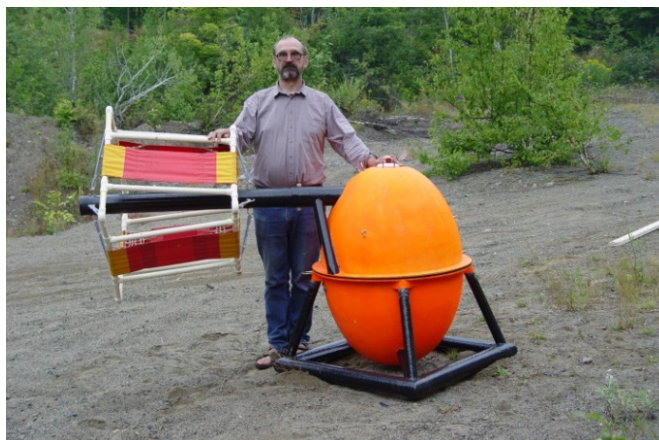
Figure 2: Geotech's airborne AFMAG system in field trials in Sudbury, Ontario with the principal designer, Dr. Petr Kuzmin. (after Lo and Kuzmin, 2004).
