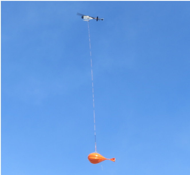
Figure 7: Helicopter MobileMT system during a survey.
