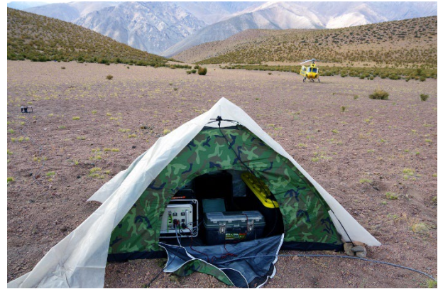
Figure 4. MobileMT electric field variations remote base station
